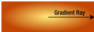
Figure 19-2. The color stops of a radial gradient are drawn on a ray extending from the center to the right
