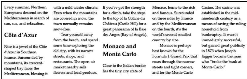
Figure 18-5. Specifying the number of columns leaves the calculation about widths to the browser
